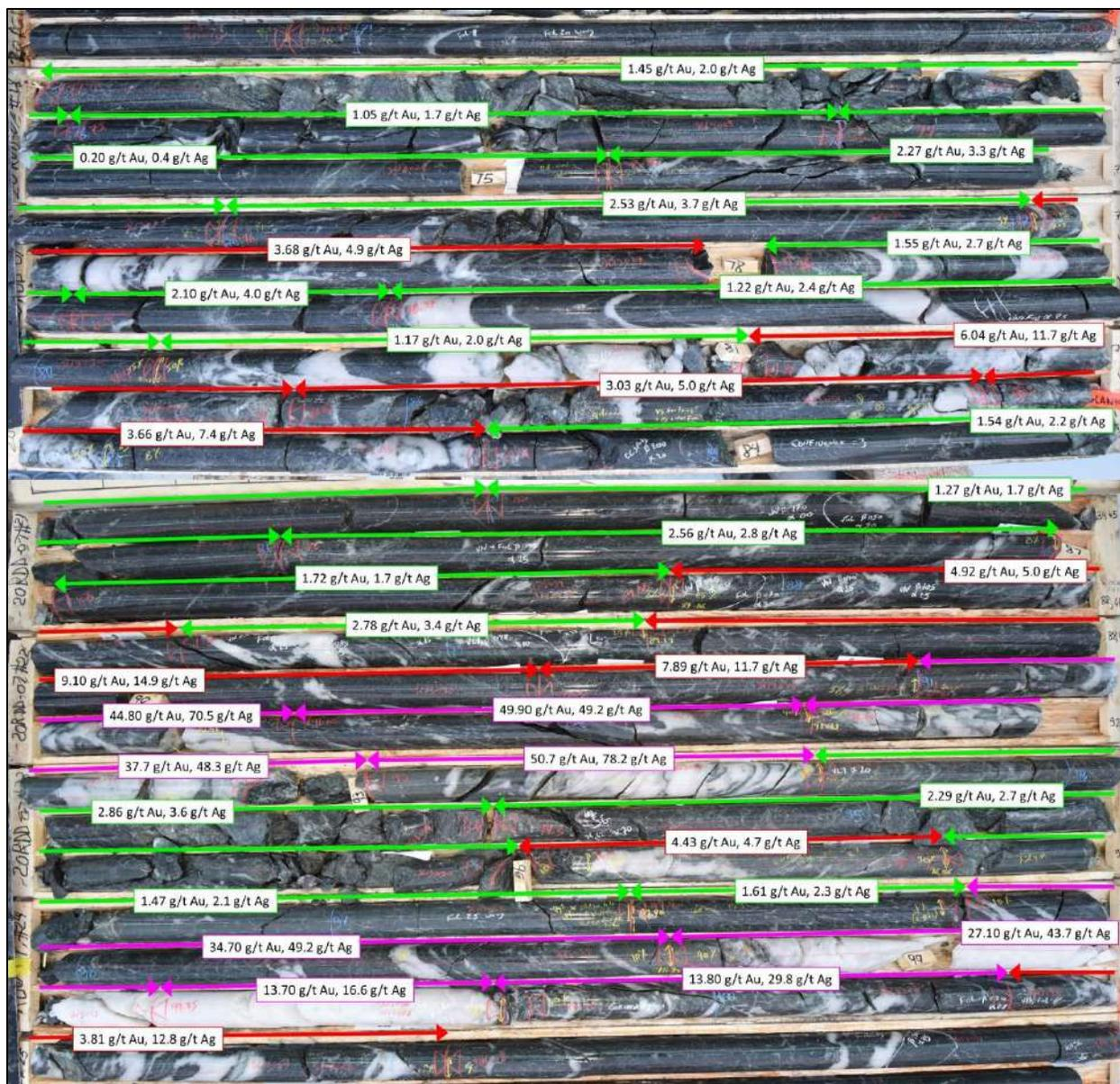
Figure 7-54: Photographs of core from drill hole 20RDD007 with gold and silver assays.
