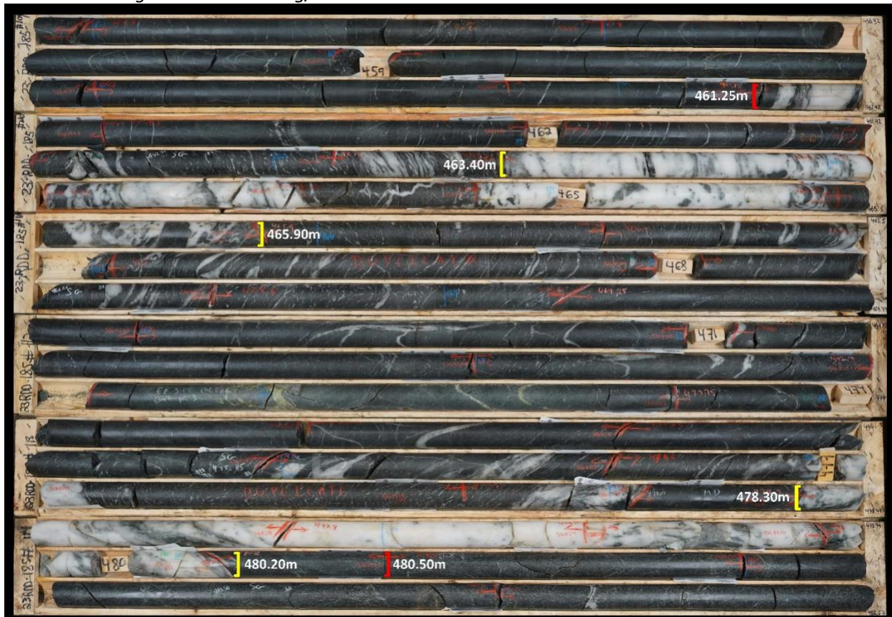
Figure 3. Core photo of R6 zone in hole 23RDD185: 19.25m at 19.95 g/t Au including 2.50m at 47.58 g/t Au and including 1.90m at 106.48 g/t Au
